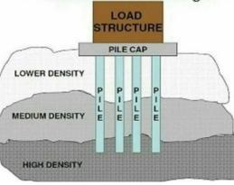
A *Pile foundation*, a kind of deep foundation, can be defined as a slender column or long cylinder made of materials such as concrete or steel which are used to support the structure and transfer the load at desired depth either by end bearing or skin friction. Pile foundations are deep foundations.
