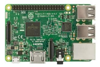
Fig .1.Raspberry Model Pi 3 Model
