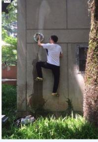
When a suction cup sticks to a rough surface rather than a smooth one, it leaves gaps that a sealing ring alone can't close tightly enough, say Kaige Shi and Xin Li, the researchers behind the new study, which was published in Physics of Fluids. Air can then escape from the outside environment into the vacuum zone, changing the pressure inside and decreasing the vacuum seal until it's completely destroyed.
