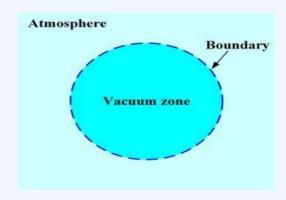
In the figure, vacuum leakage is determined by the air flow from the atmosphere to the vacuum zone, driven by pressure differences at the boundary, which is illustrated with a broken line.
