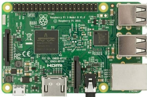
Fig .1.Raspberry Model Pi 3 Model
