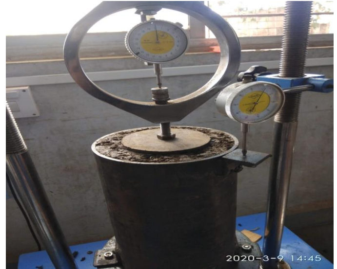
Fig 5 Stone column testing setup
