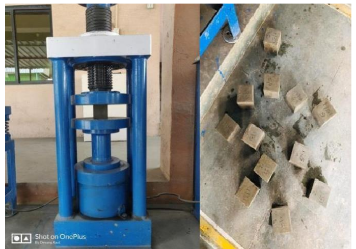
FIGURE NO : 2.2.Compressive Strength of Cubes.
