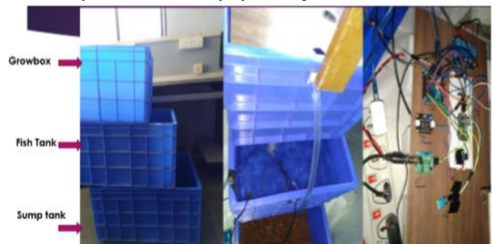
Figure 6: Implementation of aquaponics system.
