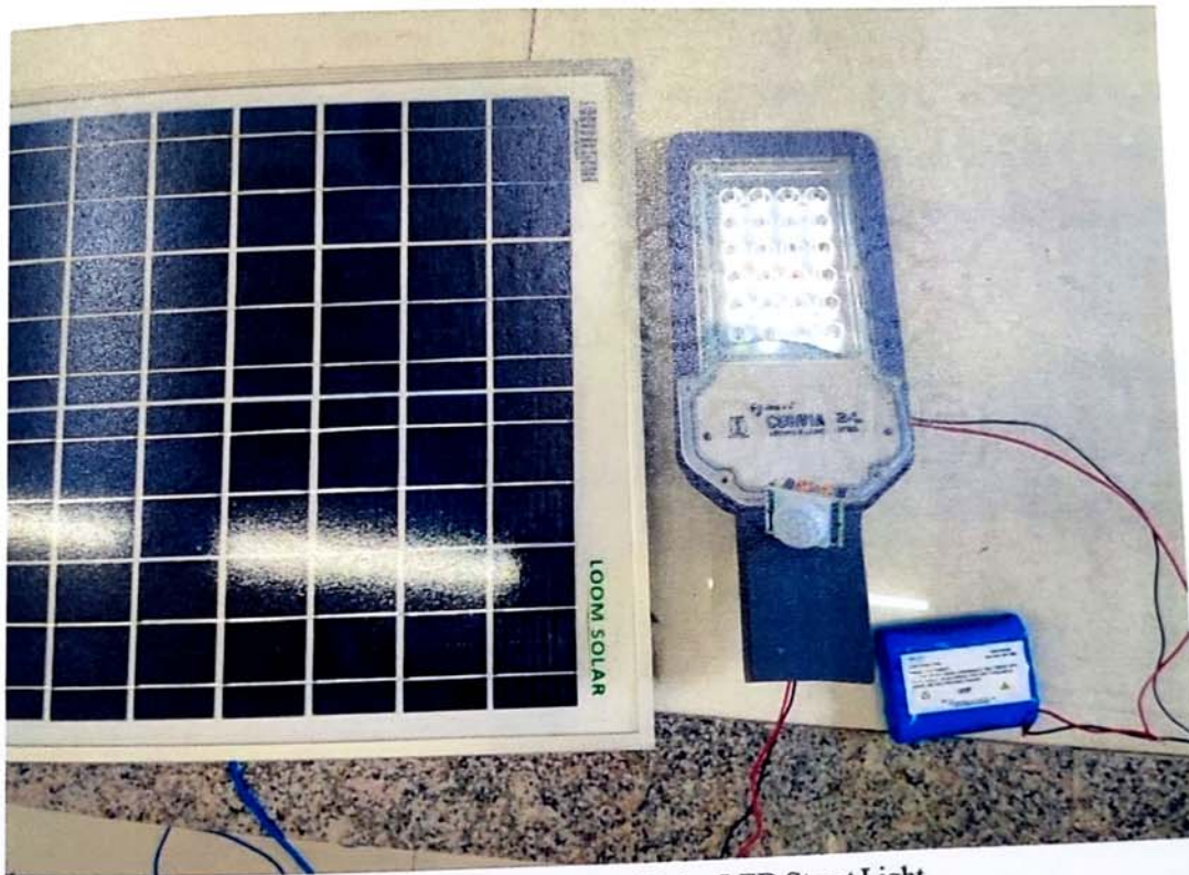
Figure 5.3: Semi-Integrated Solar LED Street Light
